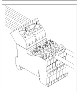
Plug the pLAN connectors into the terminals. The control circuit power can then be reconnected.
